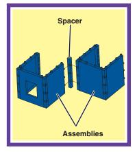
**Spacers Between Assemblies**Use a spacer to connect assemblies when needed.
