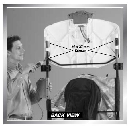
• Insert four #8 x 37 mm screws through the chute tubes, backboard tube (only the lower screws) and into the backboard. Tighten the screws.
