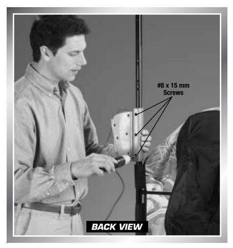
• Insert three #8 x 15 mm screws into the game selector retainer and tighten.
