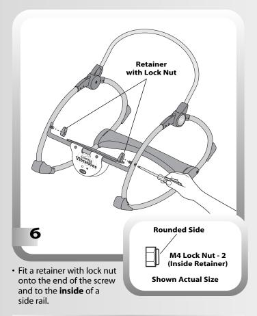
**Hint:** A lock nut has been factory assembled to the retainer. During shipment, the lock nut may have fallen out of the retainer. If it has, please fit it into the hexagonal hole in the retainer so that the rounded side of the lock nut faces out.
