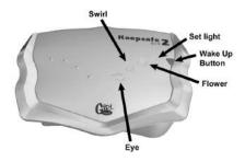
**NOTE:** If the unit will not open, remove and then re-insert the batteries (see "*Replacing the Batteries*"). This will reset the computer to the default code: Eye, Swirl, Flower. Next, repeat Step 1.
