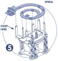
Beginning at the wide of the spiral, **"snap"** the spiral onto the posts on the quarry walls.
