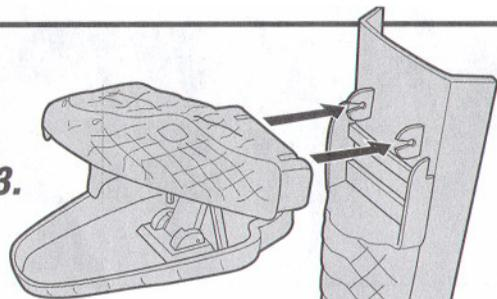
2. Slide pins under and pull up to snap into slots.
