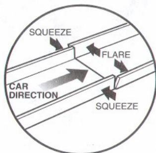
Adjust track sidewalls at each connection point as shown.
