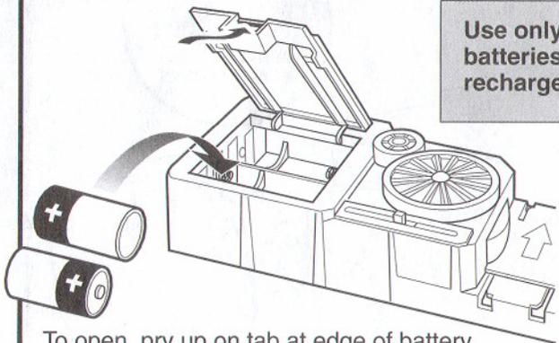
To open, pry up on tab at edge of battery door as shown. Insert two fresh "D" size batteries (not included). Close cover.
