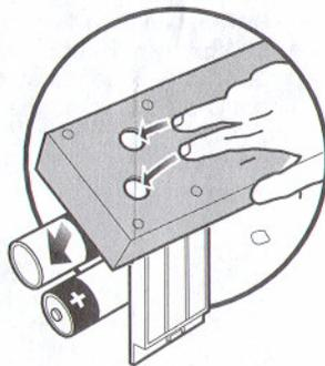
Push fingers through holes in bottom to remove batteries.
