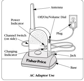
• Place the receiver where you can monitor it audibly either with or without the base. Or, wear the receiver using the convenient belt clip. Make sure the antenna points upward for best reception.
