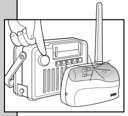
Place transmitter in room in which you intend to use it. Slide transmitter power switch to turn power on. Turn on a radio.
