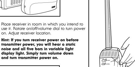
on. Adjust receiver location. Hint: If you turn receiver power on before transmitter power, you will hear a static noise and all five bars in variable light
