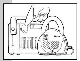
Place transmitter in room in which you intend to use it. Slide transmitter power switch to turn power on. Turn on a radio.
