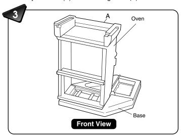
Insert the oven (A) into the rectangular opening in the base (A).
