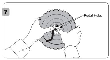
• Push the pedal hubs into the center of the front wheel until they are flush with the surface of the front wheel.
