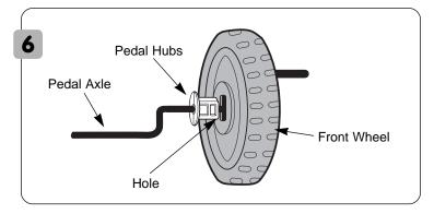
While holding the pedal hubs on the pedal axle, insert the pedal axle into the hole in the center of the front wheel.
