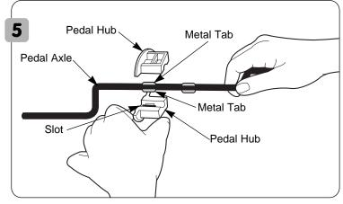
• Fit two pedal hubs onto the pedal axle metal tabs. Make sure the metal tabs fit into the slot in each pedal axle cover.
