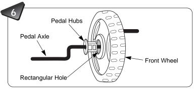
• While holding the pedal hubs on the pedal axle, insert the assembly into the rectangular hole in the front wheel.
