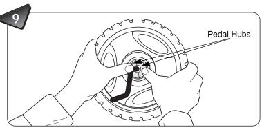
Push the pedal hubs in until they are flush with the surface of the front wheel.
