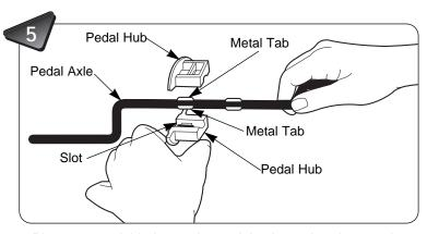
Place two pedal hubs on the pedal axle so that the metal tabs on the pedal axle fit into the slots inside each pedal hub.
