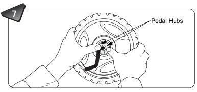
Push the pedal hubs in until they are flush with the surface of the front wheel.
