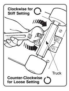
Turn Switch Board<sup>™</sup> upside-down on a flat surface. Locate both trucks (on each end).
