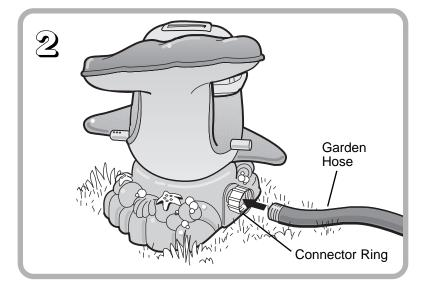
**IMPORTANT!** Before attaching a garden hose (not included) to the sprinkler, turn water on at the spigot for 30 seconds to clear debris from the garden hose. Turn water off.
