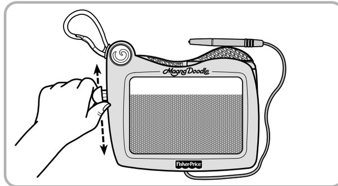
Ⓒ IMPORTANT! Before first-time use, completely darken the drawing screen with the magnetic pen. Slide the eraser lever from side to side to clear the drawing screen. Repeat this procedure several times to enable the drawing screen to create the cleanest, darkest images.
