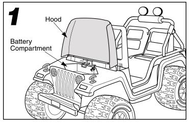
• Lift the hood to access the battery compartment.
