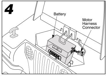
• Plug the motor harness connector into the battery. Push firmly to make sure the connectors are completely joined.
