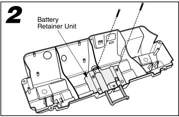
• Insert two #10 x 1" screws through the holes in the battery retainer unit and into the pegs in the dash.
