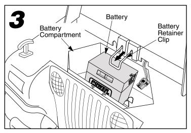
• Release the battery retainer clip. Make sure the retainer clip slides over the top of the battery. If the retainer clip does not slide over the top of the battery, reposition the battery in the battery compartment. (See step 2.)
