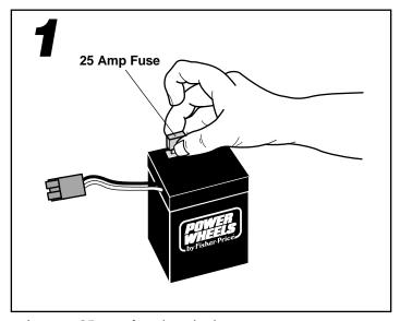
Insert a 25 amp fuse into the battery.
