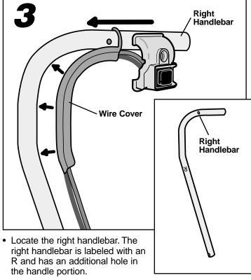
• Slide the wire cover with power button harness onto the right handlebar.
