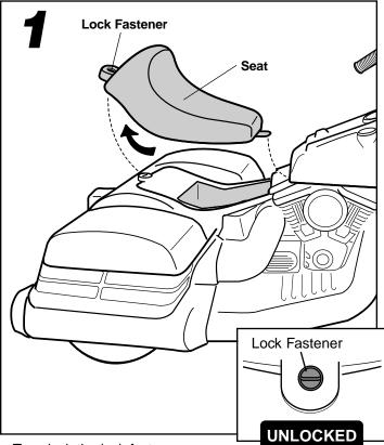
• To unlock the lock fastener, use a slotted screwdriver to rotate the lock fastener 1/4 turn to the unlocked position  $\Theta$ .
