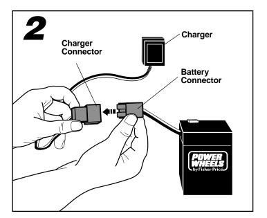
Plug the charger connector into the battery connector.
