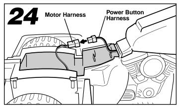
Plug the power button harness and the motor harness together. Push firmly to snap the connectors together.
