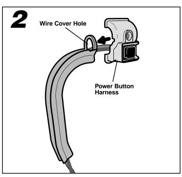
Insert the power button harness wire through the wire cover hole.
