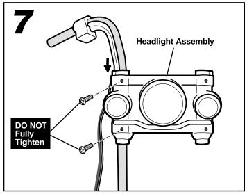
Insert two screws into the headlight assembly and hand tighten. DO NOT fully tighten these screws. These screws will be fully tightened in Assembly Step 19.
