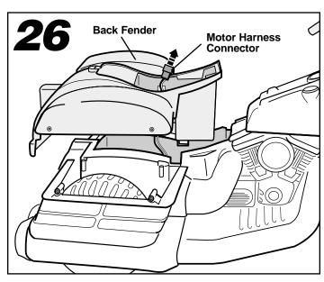
Fit the motor harness connector up through the square hole in the bottom of the back fender.
