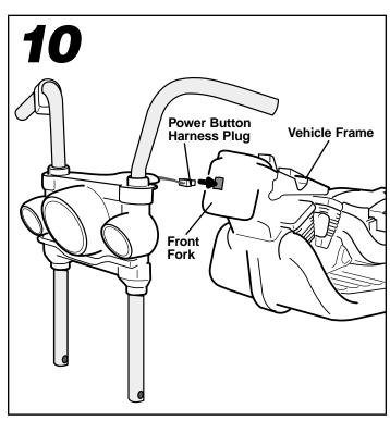
• Fit the power button harness plug through the hole in the vehicle frame front fork.
