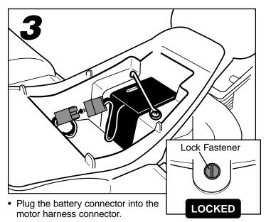
**Note:** if the battery connector will not plug into the motor harness connector, turn it over and try again! Do not force the battery connector into the motor harness connector.
