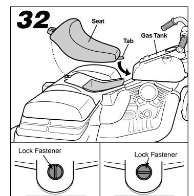
• Fit the tab on the seat into the slot in the gas tank.
