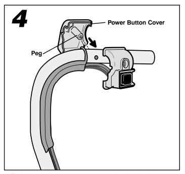
• Fit the power button cover peg into the hole in the right handlebar.
