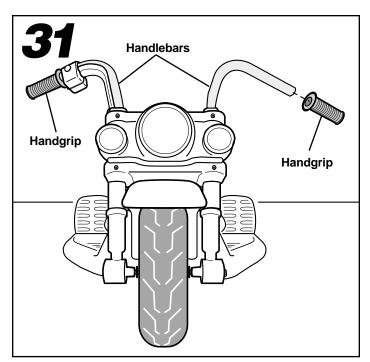
• Fit a handgrip on the end of each handlebar.
