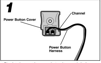
• Check to be sure the power button harness is in the power button cover channel.
