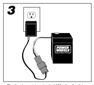
• Plug the charger into a standard 120 volt wall outlet.
