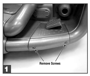
Remove the two screws in the footboard assembly.
