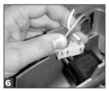
Insert the new footboard assembly black terminal into the slots in the motorcycle white connector.
