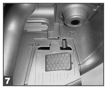
Slide the new footboard assembly back onto the motorcycle. Make sure the top (shown) and bottom (not shown) tabs insert into the slots on the motorcycle.
