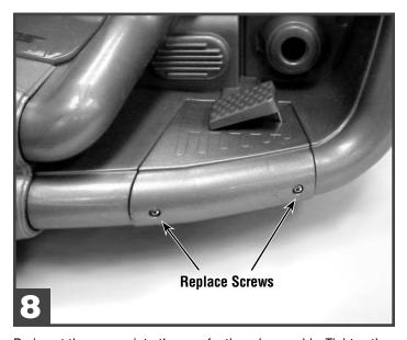
Re-insert the screws into the new footboard assembly. Tighten the screws with a Phillips screwdriver. Do not over-tighten.
