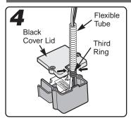
Count up three rings from the bottom of the flexible tube. Fit the notch in the black cover lid around the tube near the third ring.
