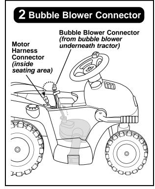
Next, connect the bubble blower connector (labeled Bubble Blower) to the second motor harness connector (labeled Bubble Blower) inside the seating area of the tractor. Please refer to Assembly steps 18 – 20 on page 12 in your Owner's Manual.
