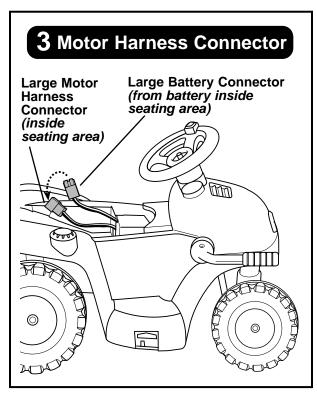
Then, connect the third, large motor harness connector to the battery connector inside the seating area of the tractor. Please refer to Battery Installation step 3 on page 15 in your Owner's Manual.
