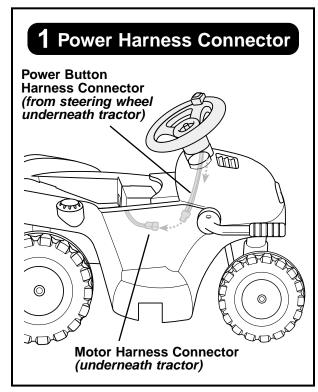
You must first connect the steering wheel power button harness connector to the motor harness connector underneath the tractor. Please refer to Assembly steps 10 and 11 on page 10 in your Owner's Manual.
