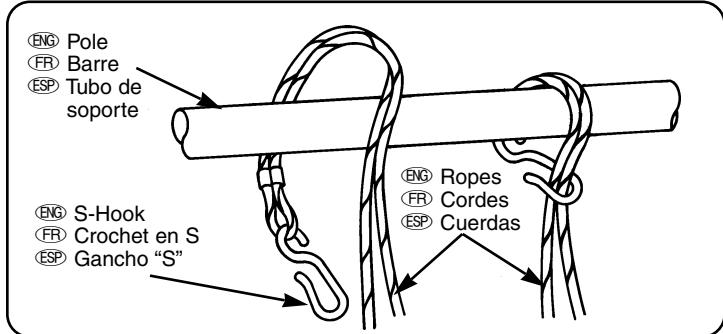
**(ENG) Please Note:** Before installing, check the strength and stability of the pole or tree branch. Place the Lift & Lock Swing at least 1 m. (3 ft.) from tree trunk or any other structure.
