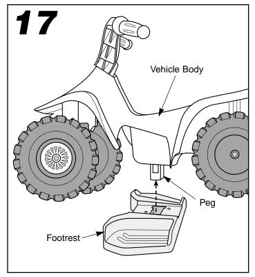
Fit the footrest to the peg on the underside of the vehicle body.
