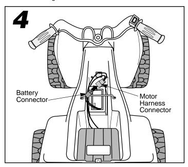
Plug the battery connector into the motor harness connector.
