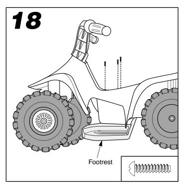
• Insert three #8 x <sup>3</sup>/<sub>4</sub>" screws through the battery compartment in the vehicle body and into the footrest.
