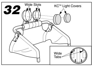
Align the four tabs on the inside of a light cover with the four slots in one of the light housings on the KC™ light rack.
