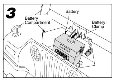
Release the battery clamp. Make sure the battery clamp slides over the top of the battery. If the battery clamp does not slide over the top of the battery, reposition the battery in the battery compartment. (See step 2.)
