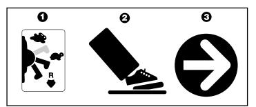
IMPORTANT! To avoid damaging the motors and gears, stop the vehicle before shifting between low and high speed.
