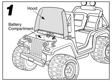
• Lift the hood to access the battery compartment.
