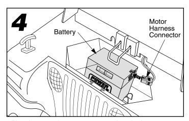
Plug the motor harness connector into the battery.
