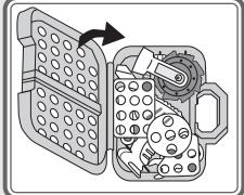
Place the remaining tools on top in the same side of the tool kit as shown above and close.
