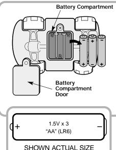
For best performance, we recommend replacing the batteries that came with this toy with new alkaline batteries.
