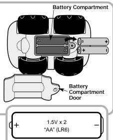
exhausted batteries from the toy. Battery leakage and corrosion can damage this toy. Dispose of batteries safely.
