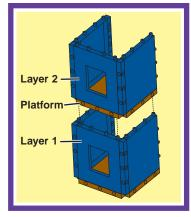
**Build Up**Build the bottom layer first, then build additional layers.
