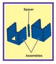
**Spacers Between Assemblies**Use a spacer to connect assemblies when needed.
