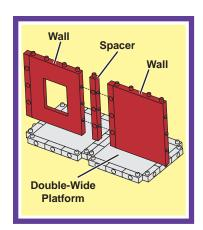
Use Spacers Between Walls that Connect to Platforms Walls joined side-by-side may require a spacer between them when connected to two single platforms, or
