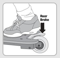
To stop the scooter, your child should press down with one foot on the rear brake, as shown.
