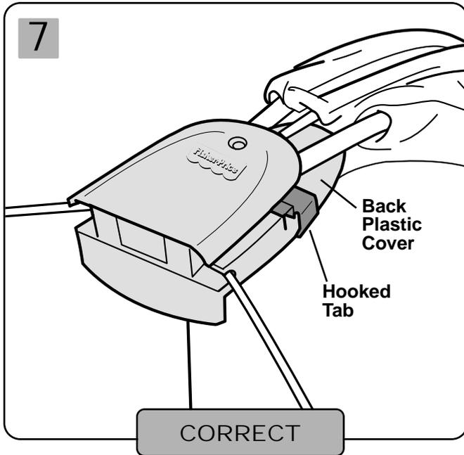
**IMPORTANT!** When correctly assembled, the hooked tabs on the bracket wrap around the back plastic cover, as shown.
