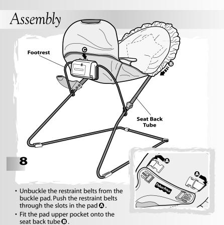
• Lift the footrest. Fit the pad lower pocket onto the footrest **G**. Lower the footrest.
