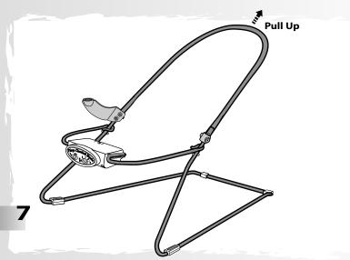
Pull up on the seat back tube to be sure it is secure. If you can remove either end of the seat back tube, you have not assembled it correctly. Remove the screws and lock nut. Re-read and repeat Assembly steps 5 – 7.
