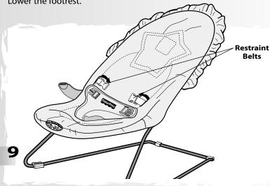
• Fit both restraint belts back through the pad slots, as shown.
