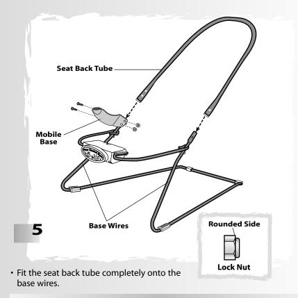
**Hint:** You will need to fit the seat back tube into the mobile base on one side of the assembly.
