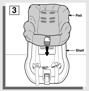
• Fit the top of the pad over the top edge of the shell.
