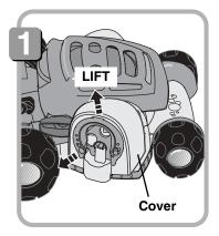
Lift up on a cover then pull it away from the mower to remove it. Repeat this procedure to remove the other cover.
