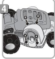
Insert the cover tabs into the slots in the mower A.
