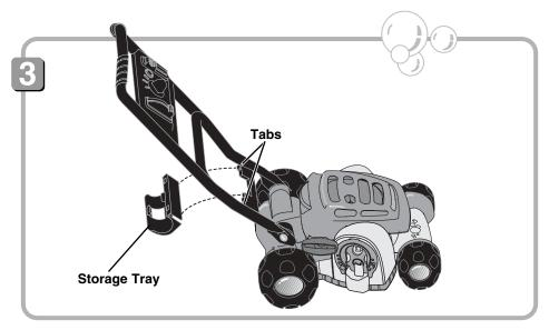
• Fit the storage tray onto the tabs on the handle. Press the storage tray until it "snaps" in place.
