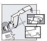
C. Still holding the spring securely, turn the chassis over.
