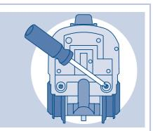
**IMPORTANT!** Under normal use conditions, the batteries in the engine will require replacement more often than the batteries in the remote controller. For additional information, see the troubleshooting section.
