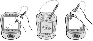
**IMPORTANT!** The mark made on your screen from the stylus and the location of the tip of the stylus may not align. When this happens, you need to calibrate the stylus.
