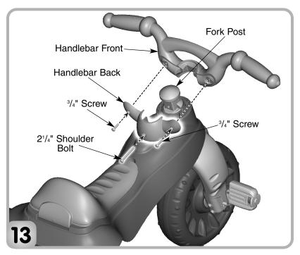
Fit the handlebar front to the fork post.
