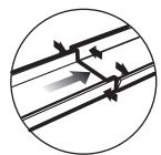
Adjust track side walls at each connection point as shown.
