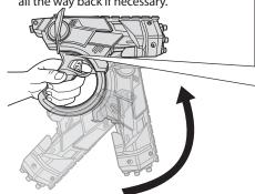
Be sure to fully charge, push or whip the barrel all the way down until "CLICK!" and the blue indicator is visible.
