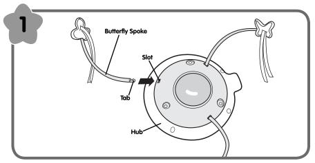
• Insert and **"snap"** the tabs on the ends of the butterfly spokes into the slots in the hub, as shown.
