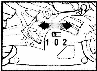
**1 - NORMAL / TEST MODE** (select this mode to test fuel performance)
