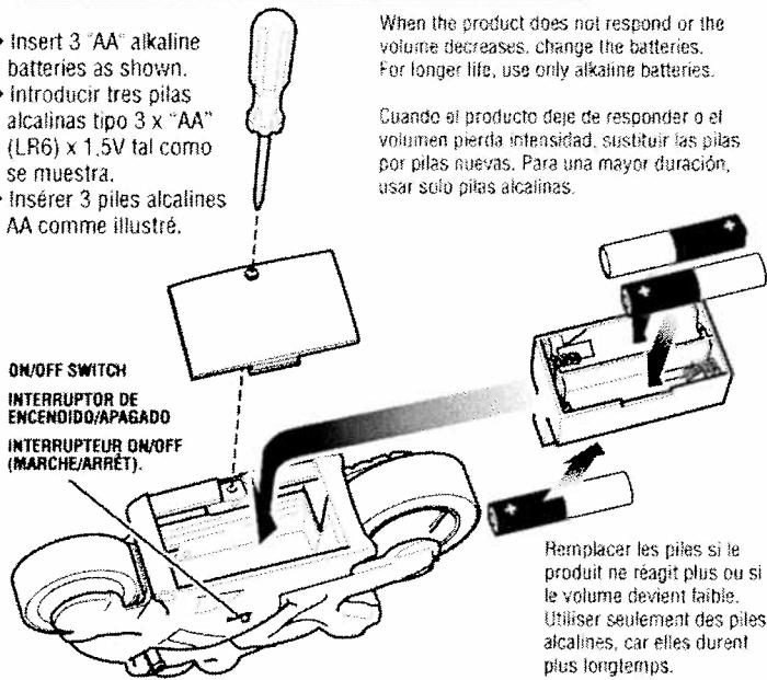
When the product does not respond or the volume decreases, change the batteries. For longer life, use only alkaline batteries.
