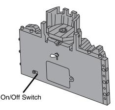
If the on/off switch is turned on  $\bigcirc$  and sounds and lights do not work, try sliding the switch off O, then on  $\bigcirc$  again.
