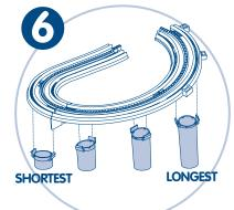
"Snap" the support pillars to the underside of the spiral track assembly, as shown, working from the shortest pillar to the longest. "Snap" the plain guardrail into the slots in the upper spiral track.
