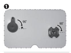
• Twist the 2 key locks found on the bottom of the package 90° and pull them out to remove the vehicle from the package.
