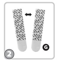
Press Command® Strip to MOUNTING BASE firmly for 30 seconds.
