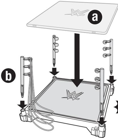
2. To attach the ropes, start from the bottom up.
