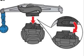
LINE UP HOUSING PINS AND CENTER HEX SLOT WITH ELEVATOR SCREW TO CONNECT.
