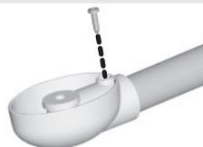
Insert two M4,5 x 1,9 cm screws. Fully tighten the screws with a Phillips screwdriver. Repeat to assemble the other feet to the other lower leg.
