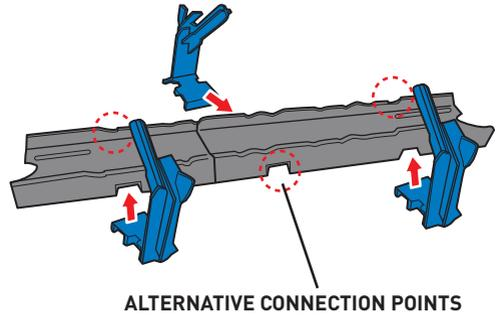
3. INSERT AND ROTATE TO LOCK ROCKET IN PLACE.
