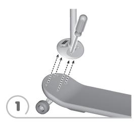
• Loosen the screws in the base of the handle and remove it from the board.
