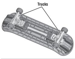
• The trucks are adjusted at the factory to the tightest setting for beginner use to provide the greatest stability. As your child becomes more comfortable and has better balance, you can adjust the trucks to a looser setting that will increase steering control.
