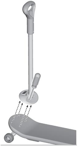
• Loosen the screws in the base of the handle and remove it from the board.
