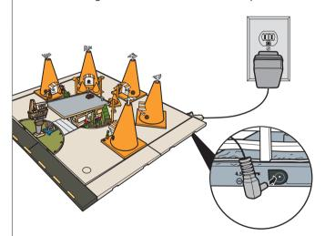
ADAPTER SPECIFICATIONS: Input voltage: 110V/220V AC Frequency: 50-60 Hz DC output voltage: 4.5 - 6V DC output current: 1000mA Plug size: 2.1mmx5.5mm jack
